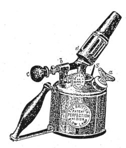
To keep the Lamp in order.—The narrow hole in the mouth-piece g must be frequently cleansed by means of the pin h (other pins or needles must not be used for this purpose, as they have a tendency to enlarge the aperture) To do this the pin must be carefully passed straight down the aperture. If the Lamp, nevertheless burns badly there must be some foreign substance in the valve opening, and to remove this, the valve c should be unscrewed, and the opening cleaned by means of the needle
