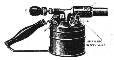
Feed the Lamp through the opening at A, and then screw on the cap TIGHTLY. Feed not more than three-fourths full. This ought never to be done near a light, or fire, nor while the lamp is burning.
