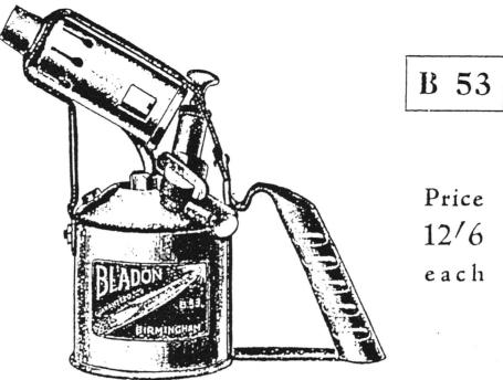
B 53. I pint, all brass, paraffin Blow Lamp, all metal handle, improved tubular Vaporizer, automatic safety device, and new design pump, extra strong make, our first model, and one we are proud of, for straight-forward work it has no equal.
