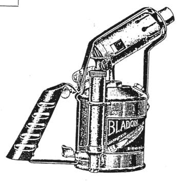
New Design Paraffin Lamp, tubular vaporizer, efficiency of flame same as Nos. B 50, B 57, B 53 and B 58. Container fitted with automatic safety device—Pump, our Patent No. 338776-29. Possesses special non-return valve operated by thumb, and controlled by coil spring. Frevents leakage of pressure or fuel. Enables lamp to be left alight and unattended without risk of fire.
