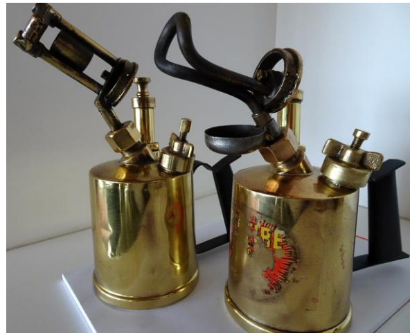
EARLY AND LATER VERSIONS OF THE VAPORISER ON A ONE-PINT (left) and TWO-PINT (right) "SPITFIRE" LAMP
