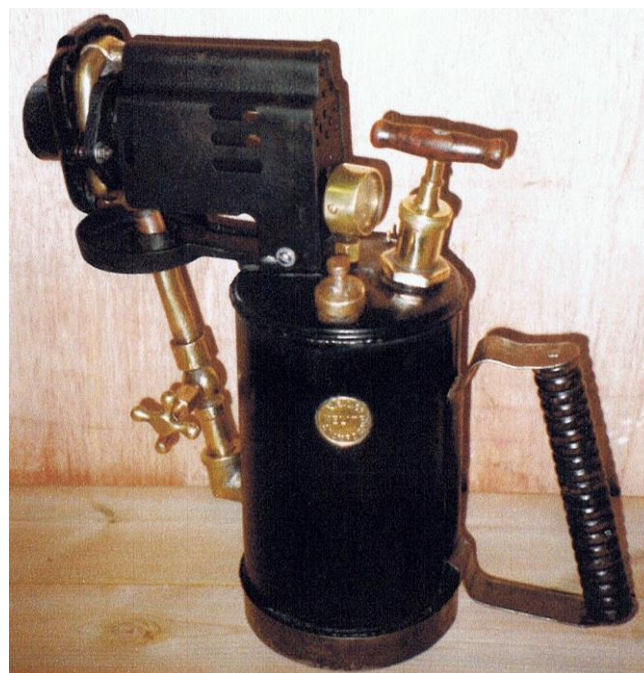
KELITE 5 Pint Paraffin Brazing Lamp. (Note the distinctive ridge around the top of the tank.)
