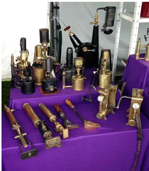
BRASS ITEMS WITH GAUGES ARE "VULCANIZERS" FOR TYRE REPAIR
