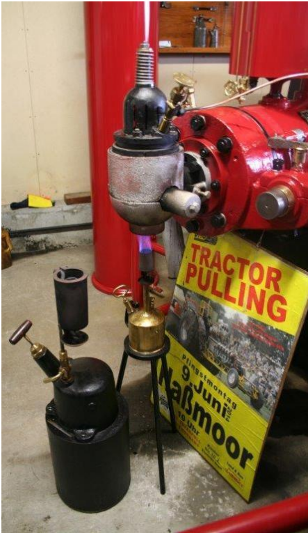
EICKHOFF ENGINE WITH PRIMUS 682 LAMP ON STAND (UNRELATED HORNSBY LAMP STANDING NEXT TO IT)
