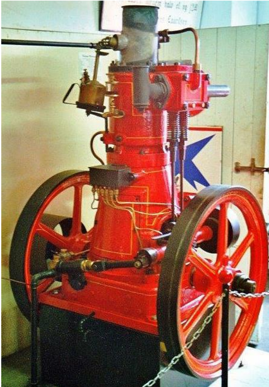
DANISH GRENA (1912) ENGINE WITH PRIMUS 682 LAMP
