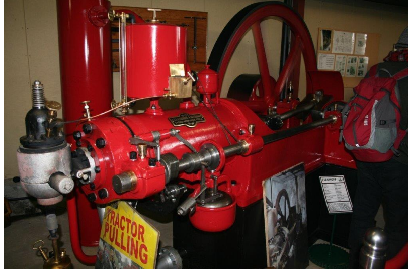
EICKHOFF ENGINE WITH PRIMUS 682 LAMP ON STAND (UNRELATED HORNSBY LAMP STANDING NEXT TO IT)
