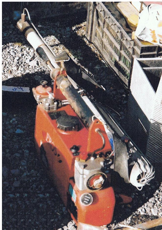
German EROS Petrol Garden Blowlamp (Editor's note: Looks to me like something out of a 1950s comic. Remember Dan Dare's Ray gun?)
