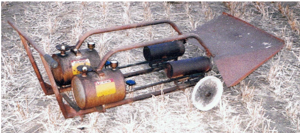
McALLAN (UK) Double Garden Burner. Each fuel tank holds 4 pints of Paraffin
