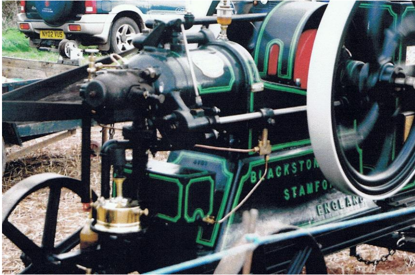
SIEVERT No. 3049 HEATER BEING USED AS A STARTING LAMP
