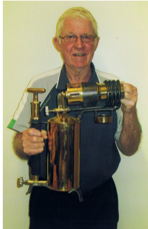
LES WITH HIS PRIMUS 866 BRAZING TORCH ABOUT 8 PINTS CAPACITY 450 MM IN HEIGHT
