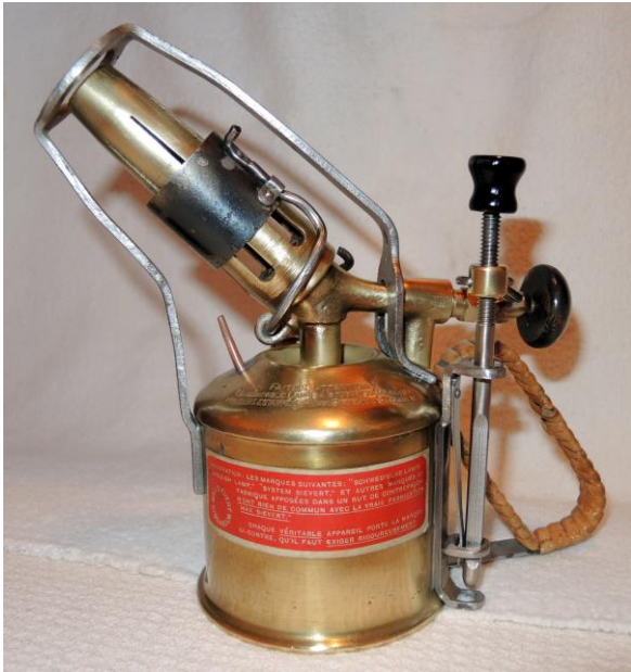
"14436 Blowlamp with a system for dimming (pilot light) just by virtue of (just by the act of) putting the blowlamp on a table or any plane surface."
