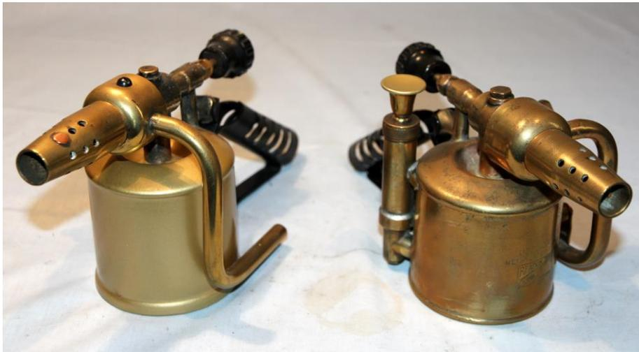
Bladon B40 Refrigerant Detector Lamps --- left: steel / right: brass
