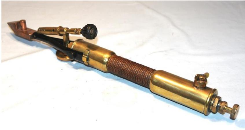
**Bladon B75 Combined Blowlamp & Soldering Iron
