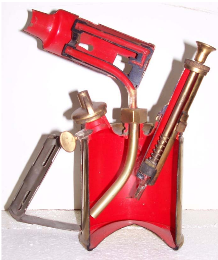
SAMUEL HEATH & SONS (UK) ONE-PINT BLOWLAMP CUTAWAY SAMPLE (Photo Bob Prichard)
