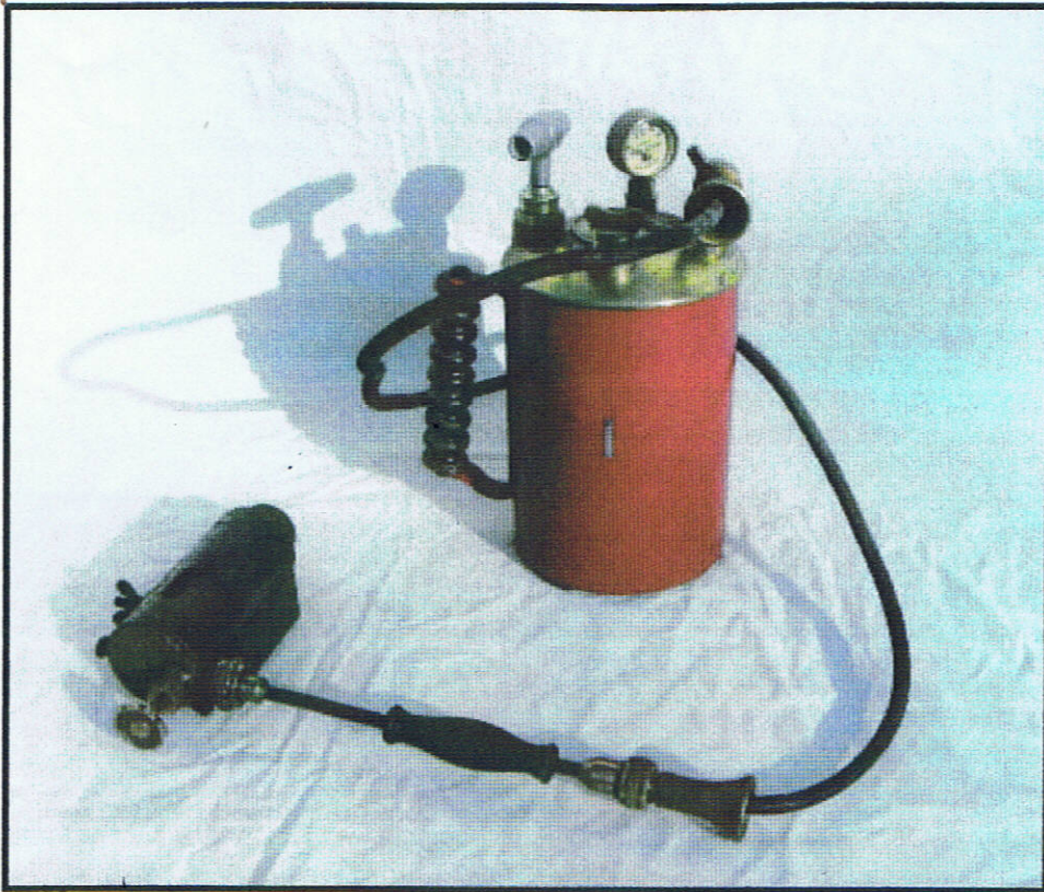
This GEM No 4, which I recently acquired from Ted Rawson, is unusual in having the flexible burner. My other GEM No4 has the usual burner fixed to the tank.
