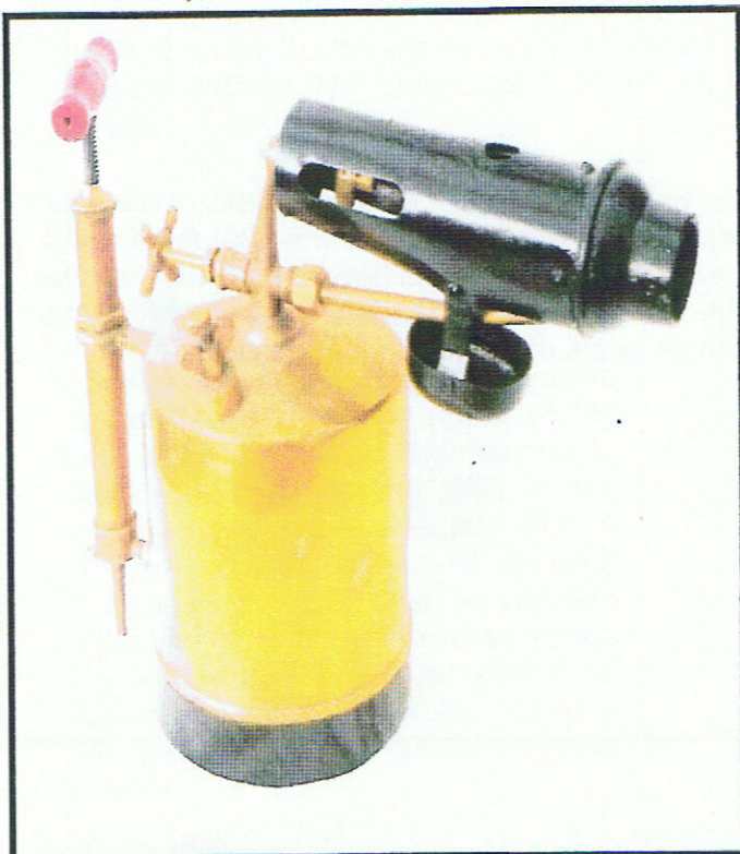
A Chinese STAR PIGEON of 2 litre capacity, a modern lamp; not rare, but with a brass tank and a pump in the handle.
