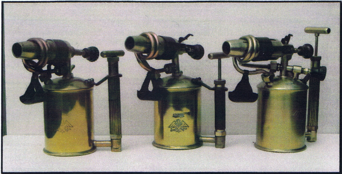
Three versions of the Mephisto 2, note the one on the right has two control valves.
