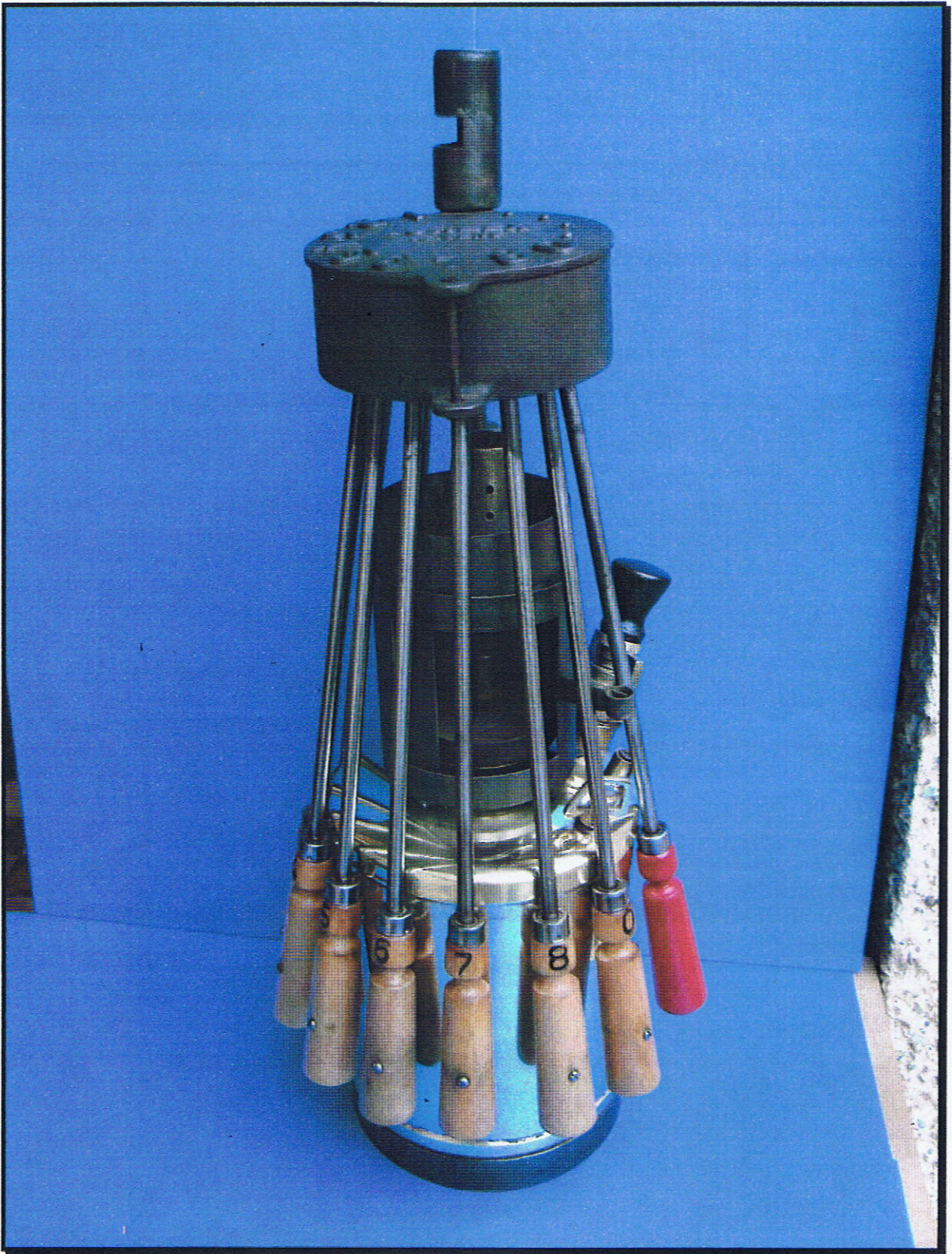
This is a most unusual blowlamp, used for heating branding irons.
