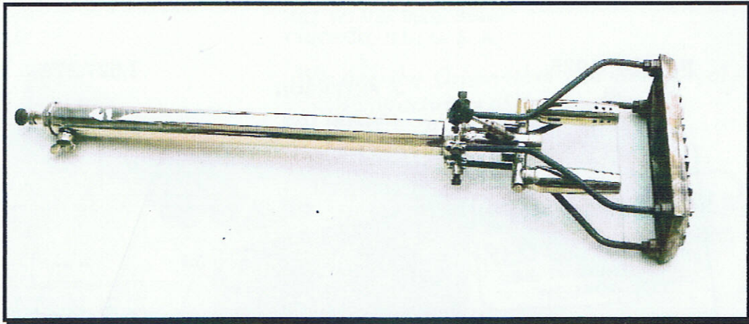
The twin burner on this model allowed for even heating of the branding plate.
