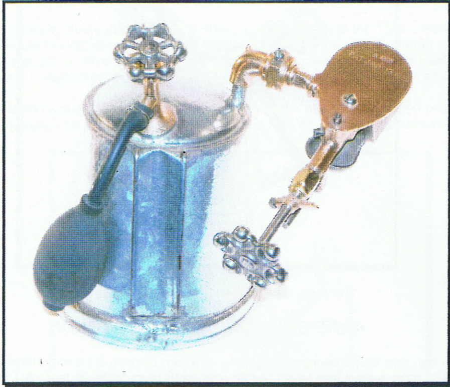
Note the rubber bulb, used to pressurise the tank.
