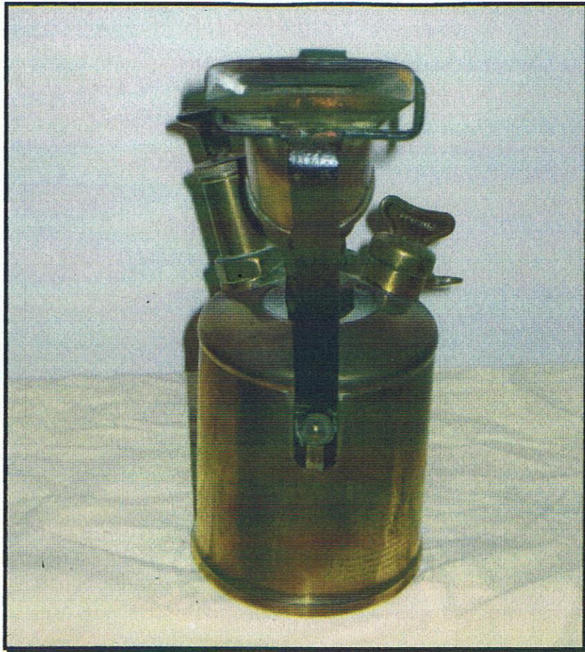
The flared burner on the Primus 655
