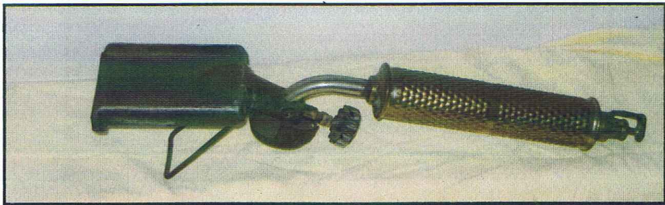
This first lamp is a Primus 951, especially made for stripping larger areas of paint.
