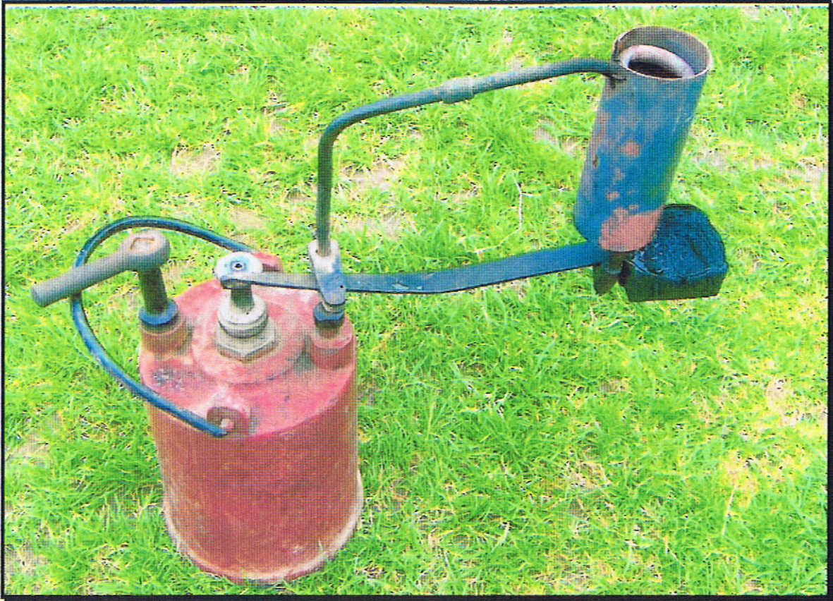
As you can see the tank is of heavy cast construction and the burner coil is not unlike that used on the Hornsby lamps.
