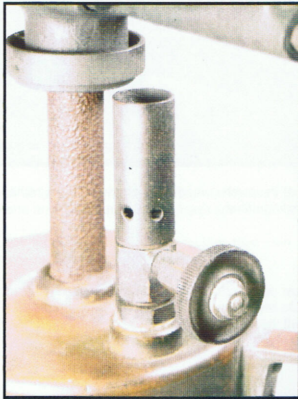
A close up of the pre-heater coming directly from the fuel tank
