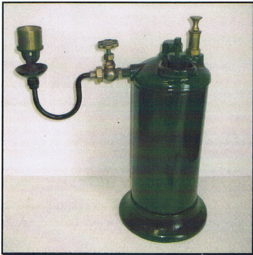
This is a blowlamp for the Campbell continuous lamp engine
