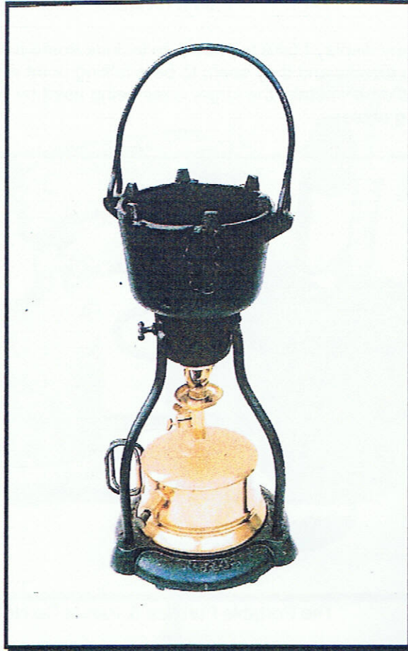
The London Furnace Co No710 made use of a Primus 702 blowlamp.
