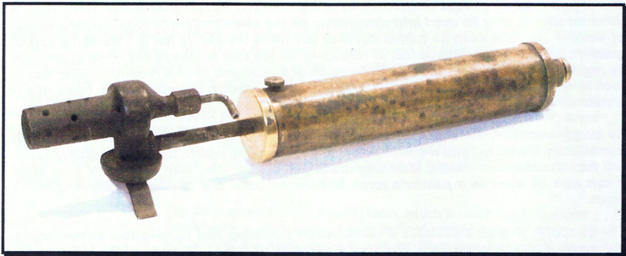
Made by the Karas Electric Co of Chicago and owned by Charles Smith. The soldering tip fixes into the end of the burner.
