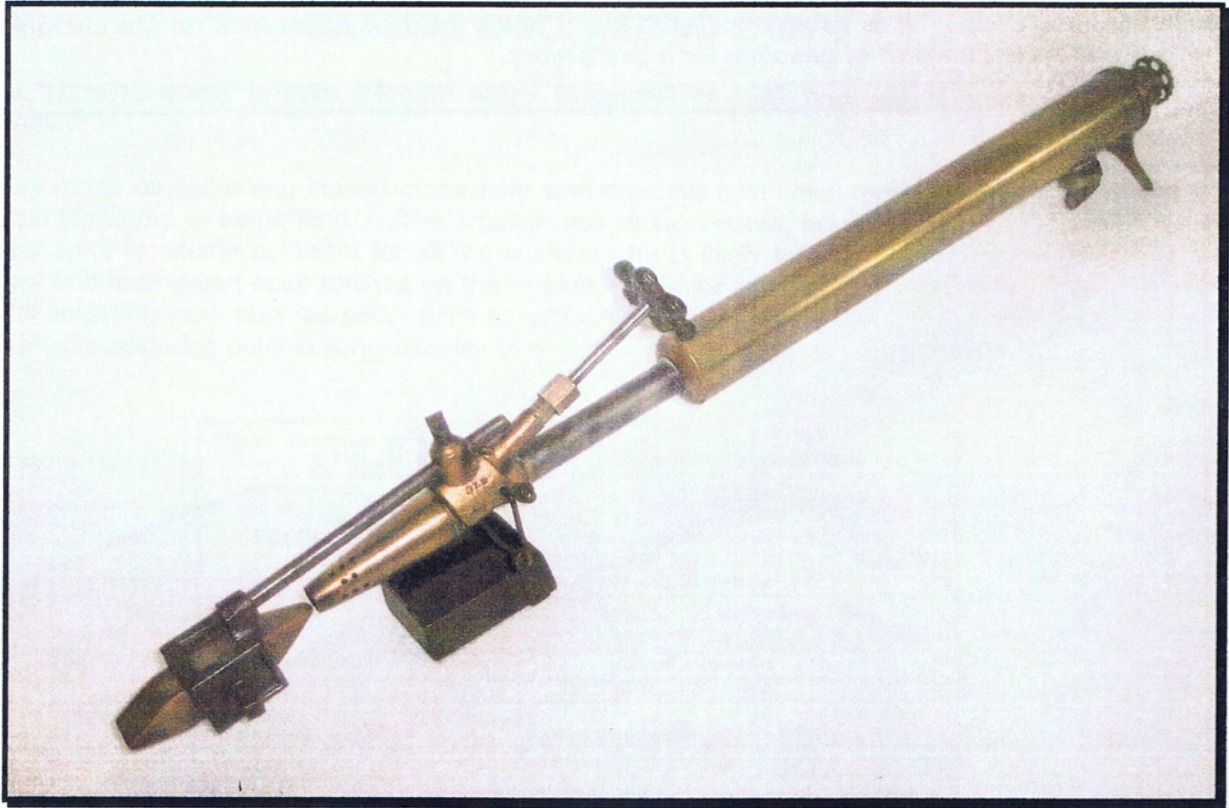
This SHSI is probably one of the largest made at over 26 inches long. It is the Otto Bernz No 75 and is owned by Ron Carr.
