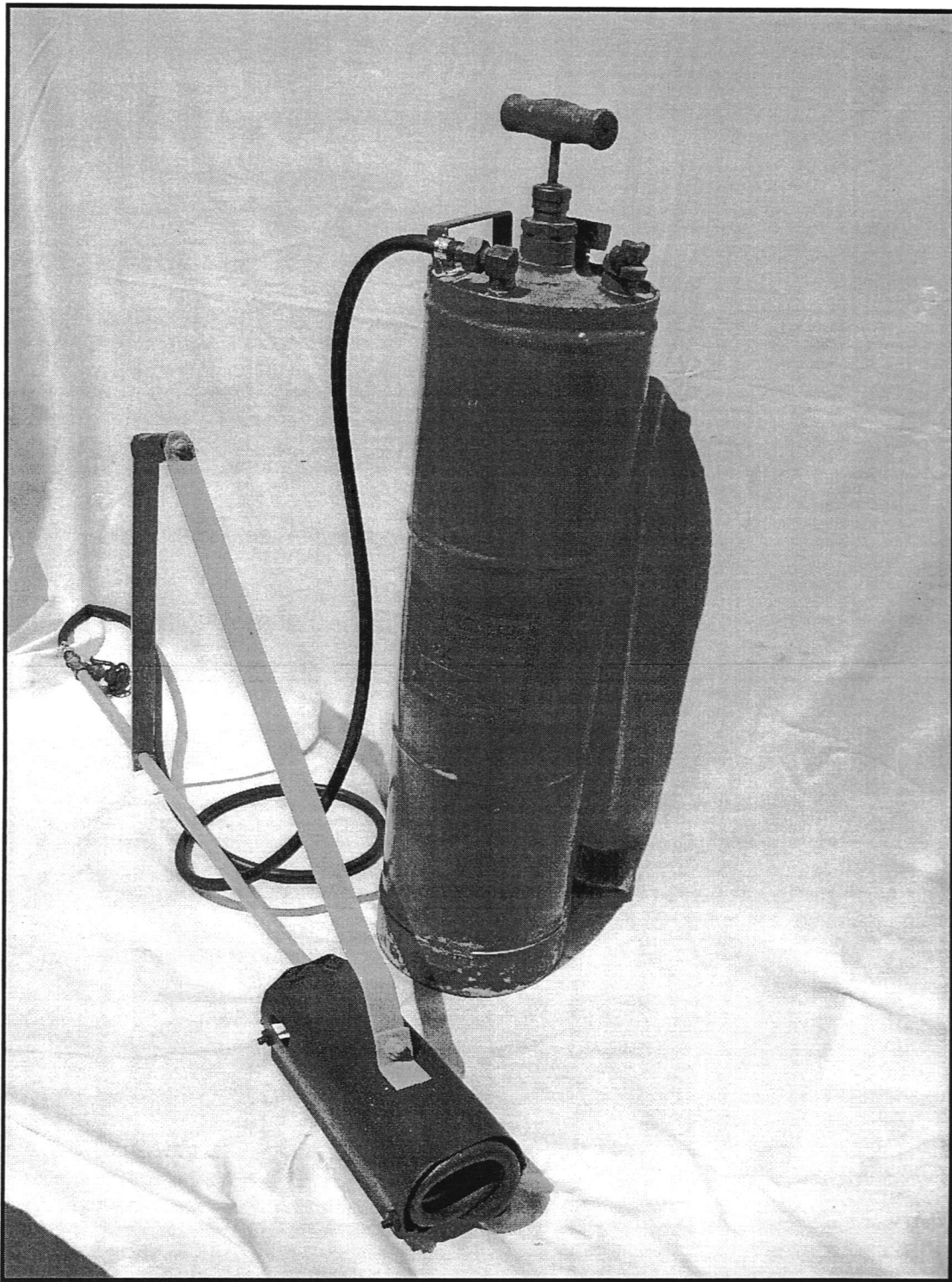
The complete flame gun, the tank is 25 inches high (63cm) by about 7 inches in diameter (18cm)
