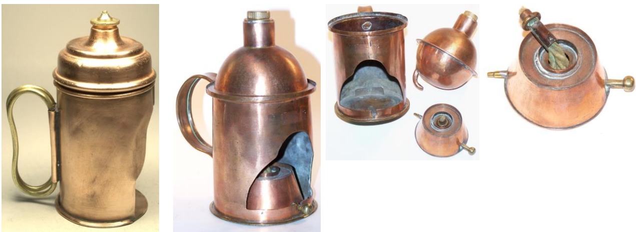
Fig. 5. Eolipyle having copper stand and brass handles, “usual” design, 15-cm high. Unmarked.
