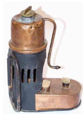
Figs. 66-68. Highly unusual Eolipyle having external front burner tube and elongate "coffin-shaped" alcohol lamp! Iron stand and handles with body bearing five vertical 28-mm by 5-mm slots on each side of stand. Rear wick on lamp heats the overlying fuel tank while the front wick serves as flame to ignite burner tip. Side filler with cork plug. Height 18-cm.
