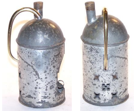
Figs. 50-52. Central 14-mm "cross" with four 12-mm "stars" at the four corners of the square-shaped cutout at back of stand (highly unusual). Stand, lower lamp, and fuel tank made of tin. Wick cap and burner tube are brass. Cork stopper in top of tank believed to be original. Note rare external loop burner tube. Unmarked. Height 14-cm.
