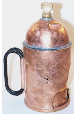
Fig. 10. Central 4-mm diameter circle plus four 2-mm diameter circles, thick copper stand 21-cm high. No pressure-release mechanism.
