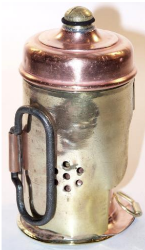
Fig. 13. Central circle with six equal 4-mm diameter circles, brass stand, slotted filler cap. Height 14.5-cm.
