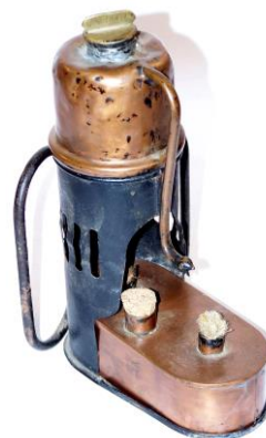
Figs. 66-68. Highly unusual Eolipyle having external front burner tube and elongate "coffin-shaped" alcohol lamp! Iron stand and handles with body bearing five vertical 28-mm by 5-mm slots on each side of stand. Rear wick on lamp heats the overlying fuel tank while the front wick serves as flame to ignite burner tip. Side filler with cork plug. Height 18-cm.
