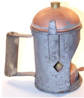
Figs. 47-48. Eolipyle with large 2-cm diamond cutout on both sides of stand. Stand, clips for fuel tank, and sheet-metal holder for wooden handle made of iron. Lower alcohol lamp and fuel container made of very thick and heavy copper. Height 17.5-cm.
