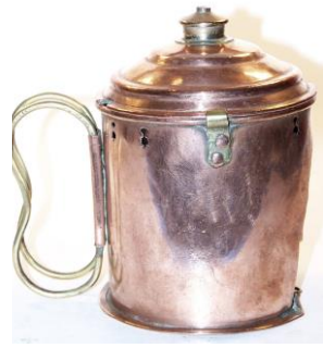
Figs. 59-60. Eolipyle with seven tiny "birds" around top of stand. Stand, lower alcohol lamp, and fuel tank are made of copper. Pull on rectangular lamp, wick cover, handles, filler plug/pressure release cap, and two clips holding fuel tank are brass. Height 15-cm.
