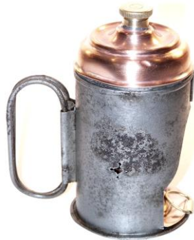
Fig. 49. Central small 5-mm diamond with tiny 2-mm diamonds at N-S and E-W quadrants. "Usual" Eolipyle, iron stand, copper tank and alcohol lamp. Height 13-cm.
