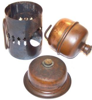
Fig. 58. Copper Eolipyle with twenty-four "keyhole"-shaped cutouts around top of stand. Pull on lower lamp, wick cap, and filler/pressure release cap are brass. Height 15.5-cm.
