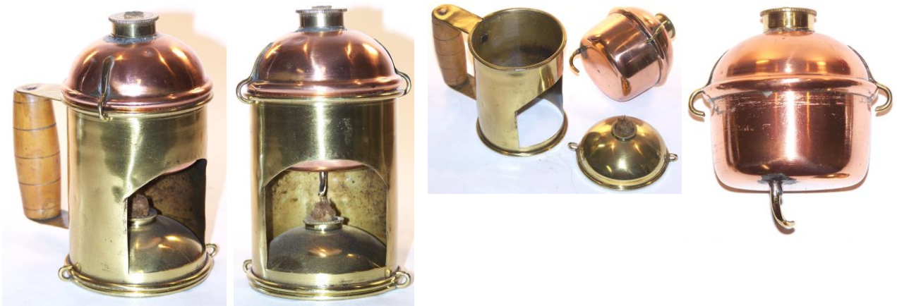
Figs. 1-4. Unusual unmarked primitive Eolipyle having no cutout on sides of stand. Brass stand with brass strap handle supports for wood handle, no bottom. Stand rests atop lower brass alcohol lamp and is fixed by two brass “hooks” fitted through slot in back rim of stand. Cylindrically-shaped copper fuel tank with two “hooks” attaches to top in similar fashion. Eolipyle is 14.5-cm in height.
