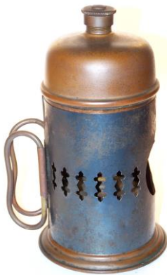
Figs. 61-62. Eolipyle having twelve vertical slot-like cutouts around the middle of the iron stand. Lower alcohol lamp and fuel container are made of copper. The loop-shaped handles, pressure release/fuel cap, and burner tube are made of brass. Height is 19-cm.
