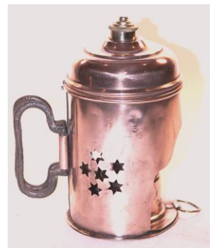
Fig. 44. Central 6-point star 13-mm wide surrounded by five identical stars. Marked "4" (size 4 Eolipyle) and "P" (unknown meaning) on base of stand. Height is 16-cm.
