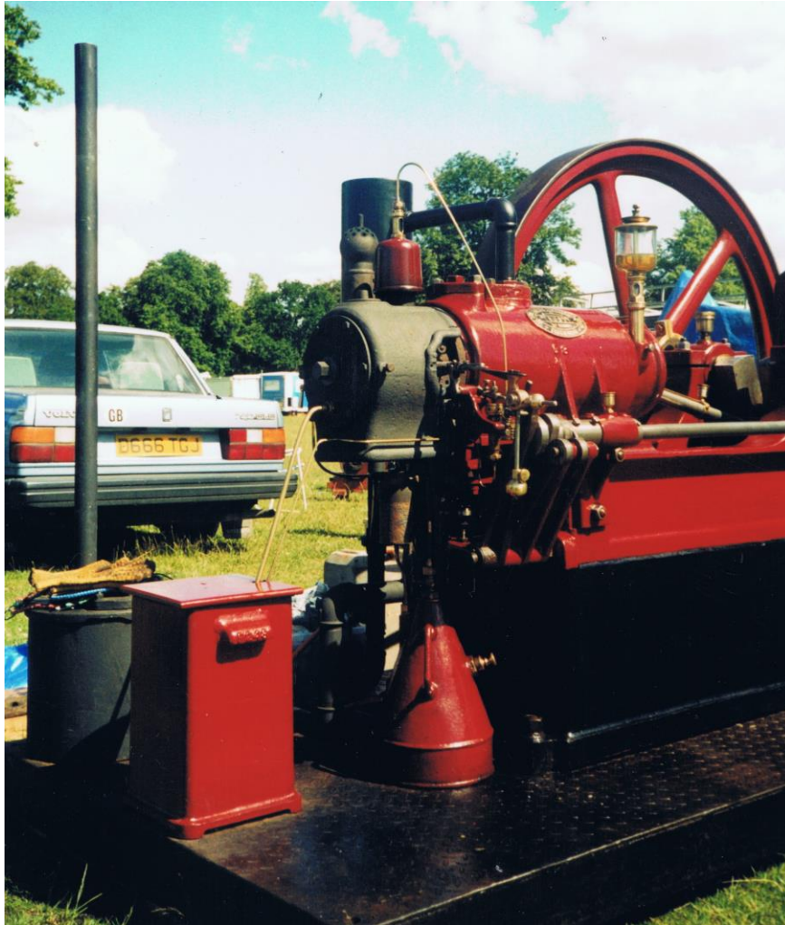
TRUSTY Engine with an unusual starting lamp
