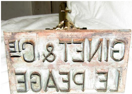
Branding plate fitted on a PHLOX 530 Made for marking the wooden barrels of a spirits distributor in south east France.
