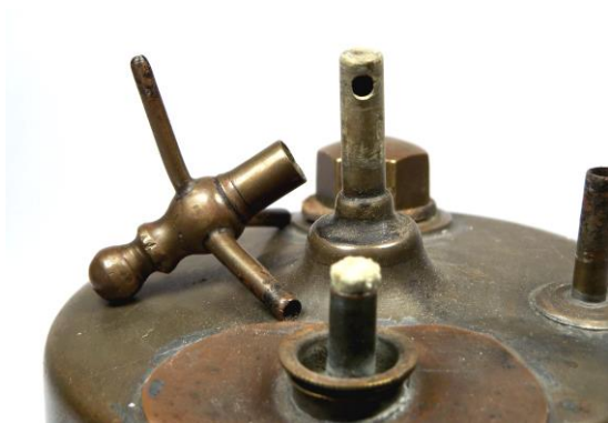
BUSH PATENT Three-way blow-pipe alcohol lamp Detail of swiveling burner (Photo Charles Smith)
