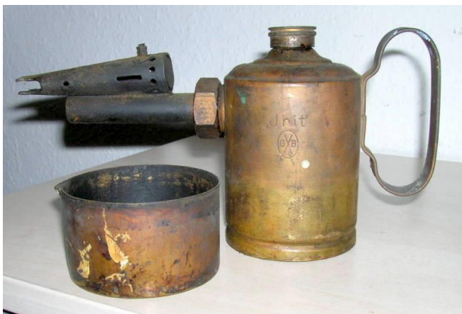
BARTHEL Model J Rit With nozzle for a Fan-shaped flame as in the above ad. item 1. Inverted, the filler cup also serves as a priming cup (Photo from Gérard MULLER.)
