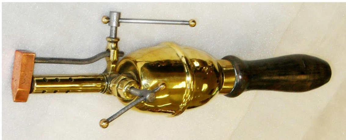
C.GOERG & CO BERLIN PAQUELIN PATENT SELF-HEATED SOLDERING IRON After 1895 Photo John Tingle
