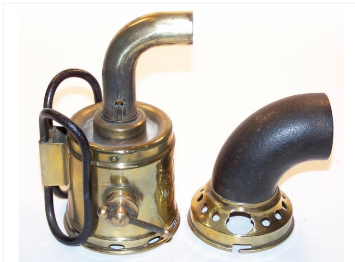
PAQUELIN No.1 LAMP, (Shown with outer tube removed. Early version with holes in the bottom flange) Photo from Charles Smith
